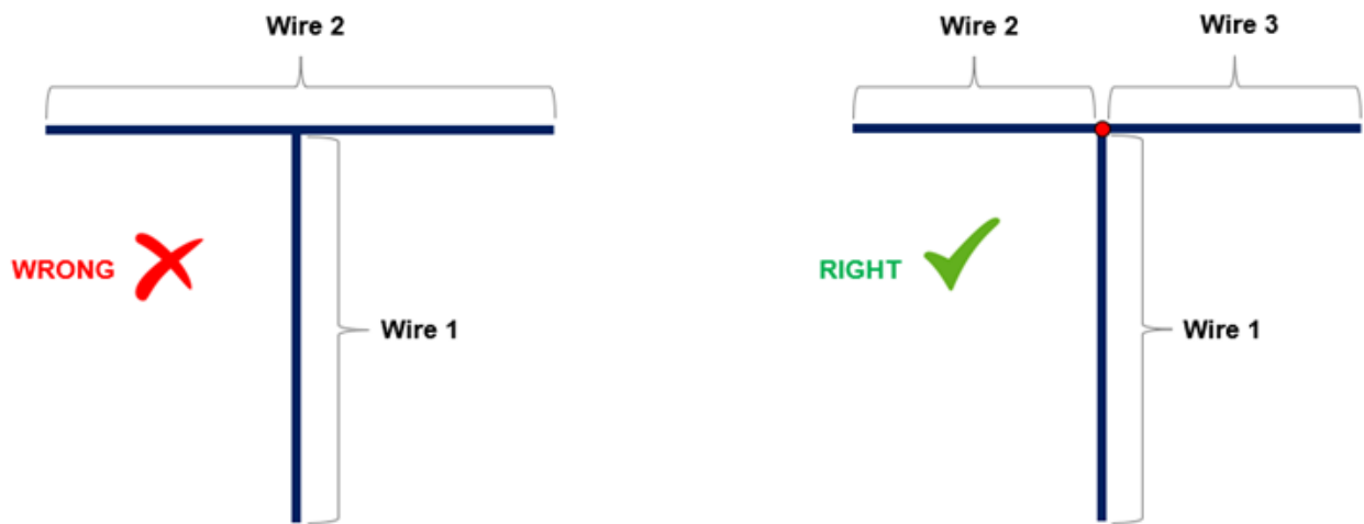
Fig. 1: Incorrect and correct methods for connecting wires.
