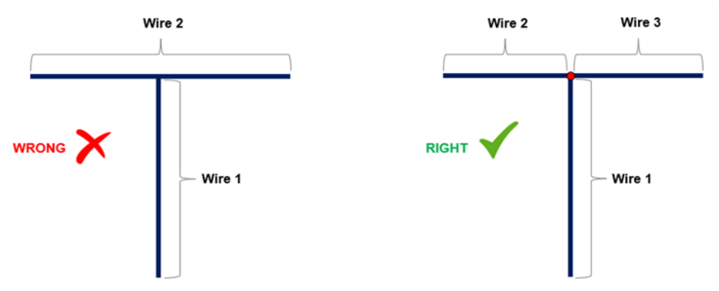
Fig. 1: Incorrect and correct methods for connecting wires.
